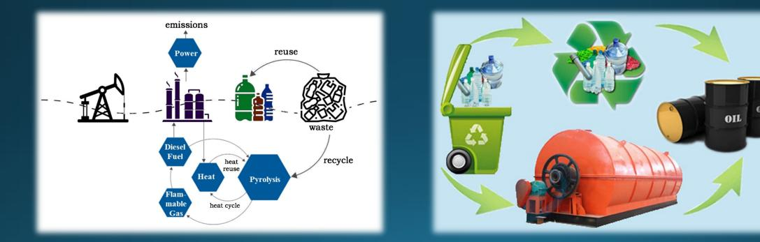
The basis of the developed technology, like other similar ones, is low-temperature controlled pyrolysis of polymers without air access in the presence of catalysts.
